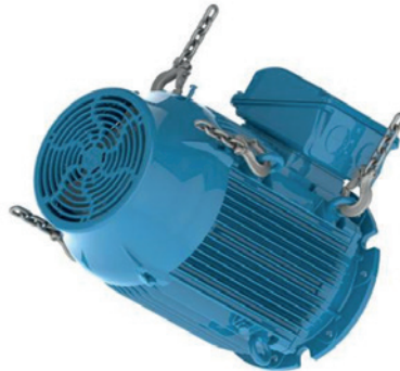
Figure 4.19 - Motor is being rotated to horizontal position
